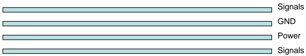
Figure 12: Typical 4-layer PCB construction
